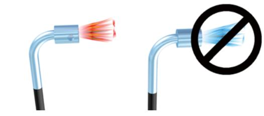
Use yellow/orange flame when heating RW material. Blue flame will overheat material.
