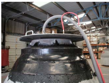
Riser-Wrap® Vacuum Test
