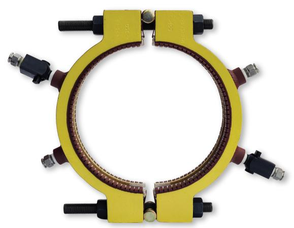
Plidco<sup>®</sup> Flange+Repair Rings can be installed by your own personnel. There is no drilling or altering of flanges. On a scheduled turnaround the Plidco<sup>®</sup> Flange+Repair Ring can be reconditioned and used again. Give us your conditions — pressure, temperature, fluid — and we will recommend the proper sealant and packing. Standard packing is non-asbestos aramid fiber.
