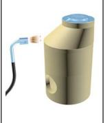
2. Preheat manhole surface. The function of preheating is to remove excess moisture.
