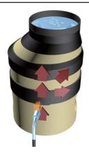
**6.** Using a moderate to high flame, begin heating Riser-Wrap® sleeve material from the bottom edge moving around the structure in one direction.
